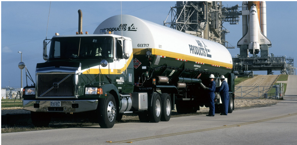
Figure 5: Liquid hydrogen tanker of 25 000 l
