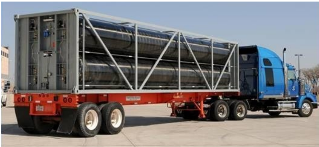
Figure 6: Composite tube trailer of 25 000 l of gaseous hydrogen at 250 bar.
