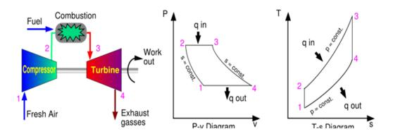
2. The efficiency of the cycle is the ratio between what we are interested in (net work provided by the gas on the shaft, ie  $\Delta H_{12} + \Delta H_{34}$ ) to the heat provided to the system  $Q_{23}$ . Over the cycle,  $\sum \Delta H_i = 0$  and  $\Delta H_{23} = Q_{23}$  and  $\Delta H_{41} = Q_{41}$  so
