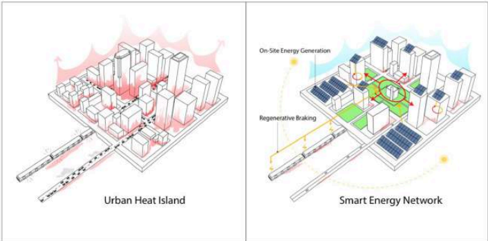
Figure 4 Typical and best practice scenario for energy uses in a district (NYIT Urban Climate Lab, 2017)
