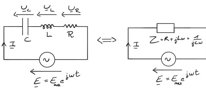
$$\underline{E} = Z\underline{I} \implies \underline{I}(t) = \frac{E_{\text{max}}}{\left(R + jL\omega + \frac{1}{jC\omega}\right)} e^{j\omega t}$$
