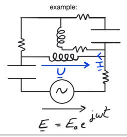
$$\underline{U}(t) = \underline{U}_0 \, e^{j \underline{\omega} t} \, _{\text{the generator}}$$
