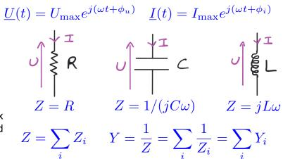
Forced RLC circuit: resonance when it is excited at the natural oscillation frequency of the circuit.
