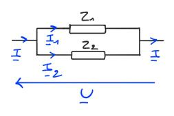
$$\underline{I} = \underline{I}_1 + \underline{I}_2 = \frac{1}{Z_1}\underline{U} + \frac{1}{Z_2}\underline{U} = \frac{1}{Z}\underline{U}$$
