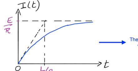
The current in the coil is established with a characteristic time L/R
