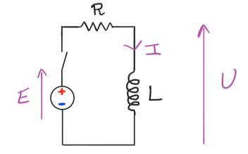
Initially I=0, and at t=0 the switch is closed.
