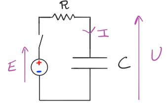
Initially U=0, and at t=0 the switch is closed.
