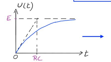
The capacitor is charging to E with a characteristic time RC
