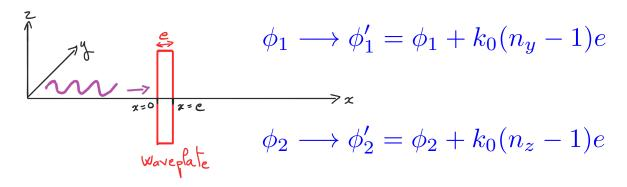
How to determine the form of the wave after a waveplate of thickness e?
