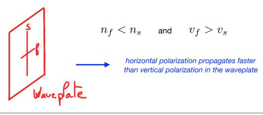
How to determine the form of the wave after a waveplate of thickness *e*?
