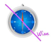
no current in wire (I=0), magnetized needle points North
