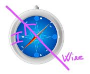
current in opposite direction, needle switches direction
