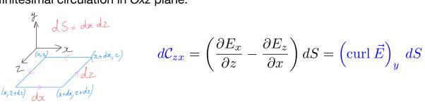
The component of the curl along a given axis is the circulation along an infinitesimal loop in the perpendicular plane per unit area
