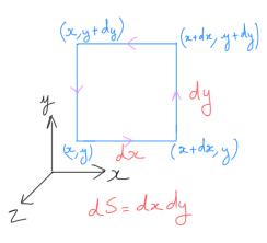
Bottom side:  $\vec{E} \cdot \vec{dl} = E_x(x, y, z)dx$ Top side:  $\vec{E} \cdot d\vec{l} = -E_x(x, y + dy, z)dx$
