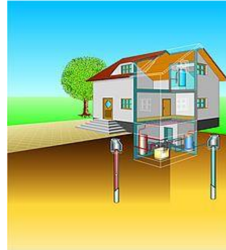
Water source heat pumps
